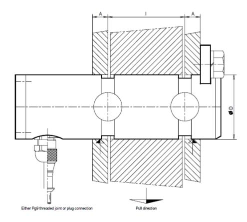
The Load Pin must be embedded in a smooth running but free of mechanical play in the inner bearing and lubricated.
